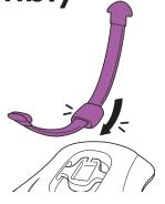
Insert the front of the central rail into the grooves in the front of the rocking trolley. Then push the rail down until you hear a click.
