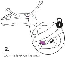
Lock the lever on the back of the rocking trolley.
