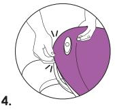
Pull the seat fabric over the toy bar opening and snap into place.
